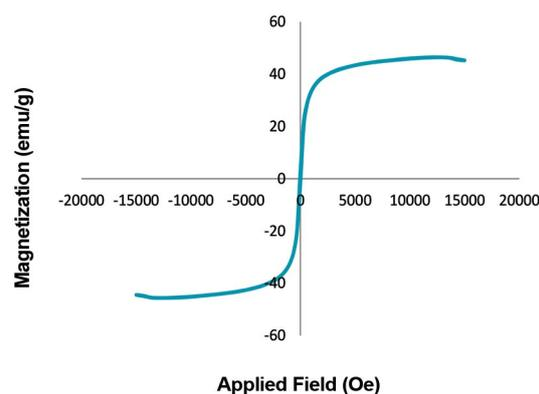
Fig. 6. Hysteresis loop of NiFe<sub>2</sub>O<sub>4</sub>/sawdust at room temperature.
