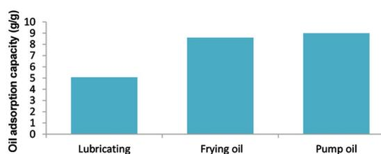
Fig. 7. Oil adsorption capacity of NiFe<sub>2</sub>O<sub>4</sub>/sawdust magnetic nanocomposite for three types of oil.
