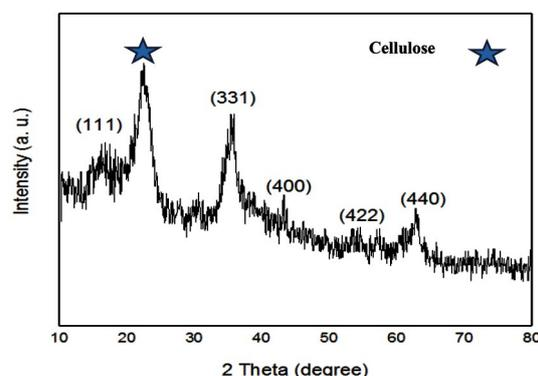
Fig. 3. XRD pattern of NiFe<sub>2</sub>O<sub>4</sub>/Sawdust nanocomposite.
