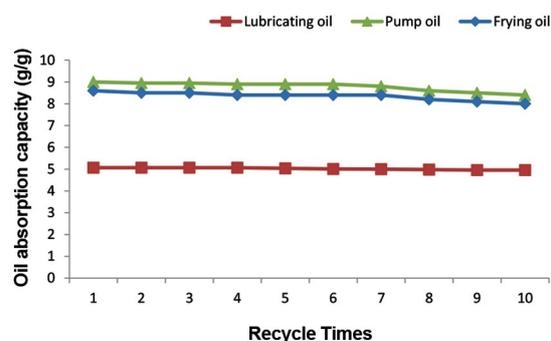
Fig. 8. Oil adsorption capacity of modified sawdust for three types of oil after 10 oil removal cycles.
