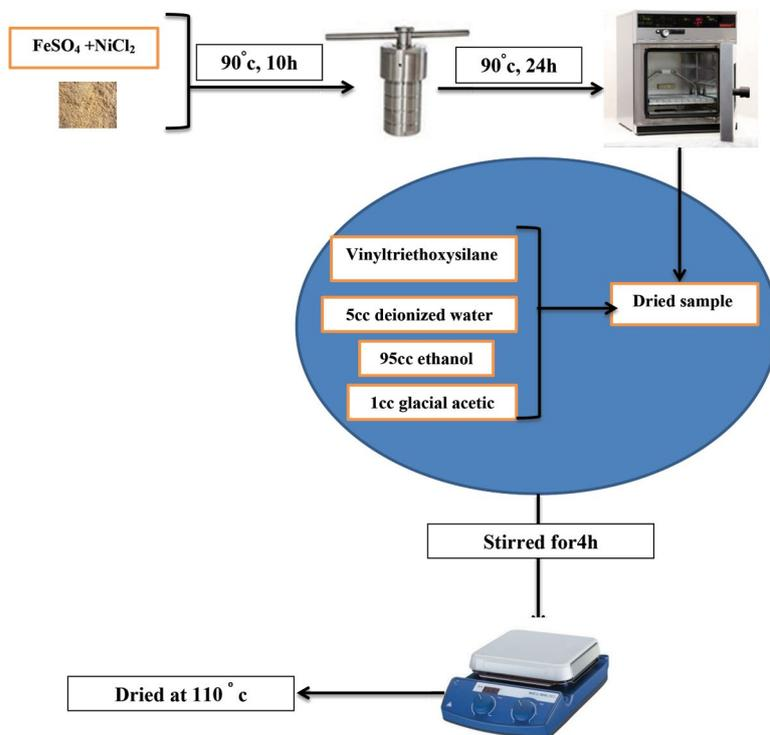
Fig. 1. Illustration synthesis procedure of NiFe<sub>2</sub>O<sub>4</sub>/sawdust nanocomposite.
