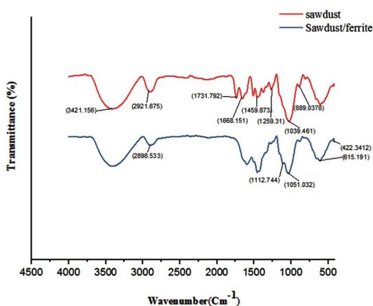
Fig. 4. FTIR spectrum of sawdust and NiFe<sub>2</sub>O<sub>4</sub> /Sawdust nanocomposite.
