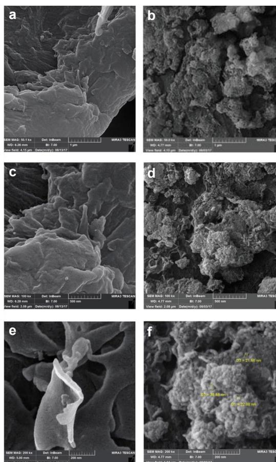
Fig. 5. a. c. e FESEM image of raw sawdust b. d. f NiFe<sub>2</sub>O<sub>4</sub> /sawdust nanocomposite.
