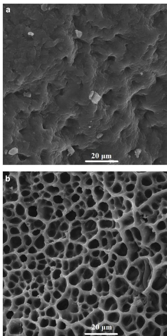
Fig. 5. SEM images of PAA/OVS hydrogel before (a) and after swelling (b).
