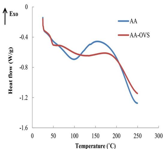
Fig. 6. DSC curves of the AA and AA-OVS hydrogel.
