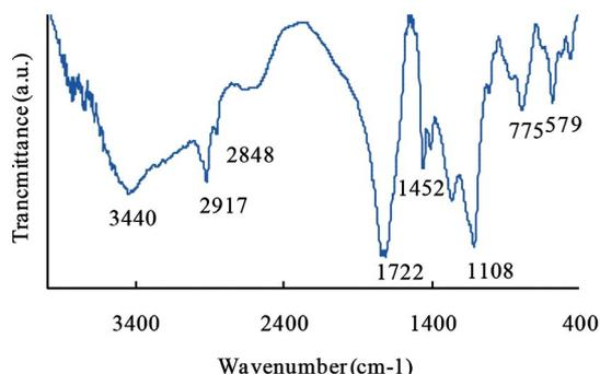
Fig. 7. FTIR spectrum of the PAA/OVS nanocomposite hydrogel.
