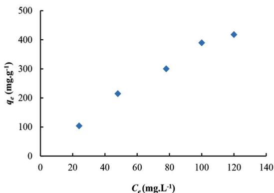
Fig. 10. Effect of initial dye concentration on the adsorption of MB dye by PAA/OVS hydrogel.
