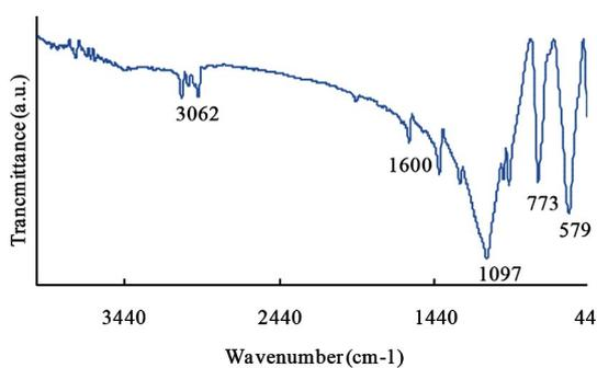
Fig. 4. FTIR spectrum of the OVS.
