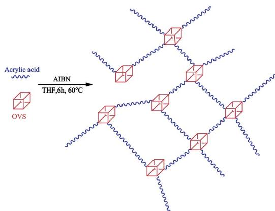
Fig. 1. Schematic representation of the preparation of crosslinked PAA/OVS organic-inorganic nanocomposite hydrogel by radical polymerization.
