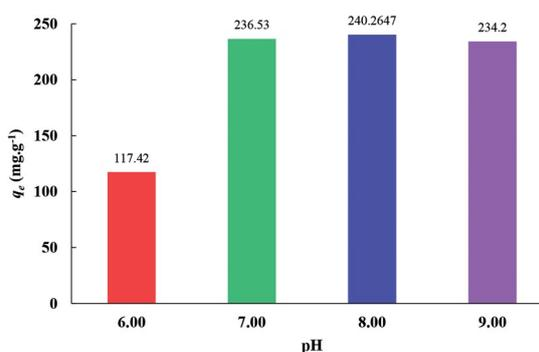
Fig. 8. variation of adsorption capacity of the PAA/OVS hydrogel for MB at different pH ( $100 \text{ mg} \cdot \text{L}^{-1}$ ).
