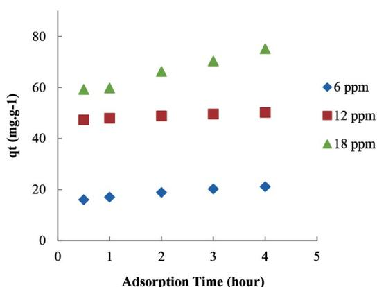
Fig. 9. Effect of contact time on the adsorption capacity.
